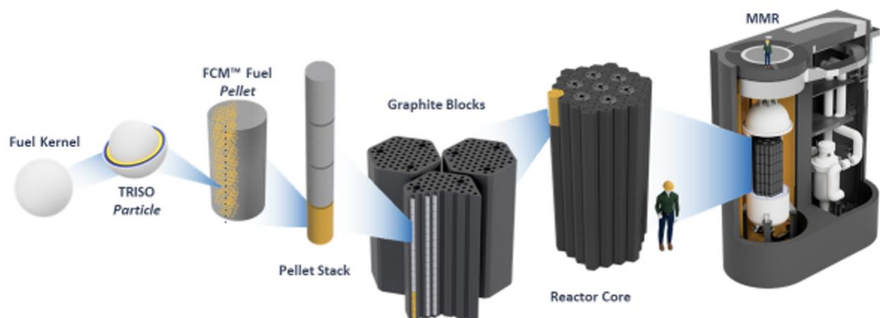
Figure 26: Conceptual arrangement of the MMR core consisting of TRISO particles, FCM fuel and graphite blocks.
