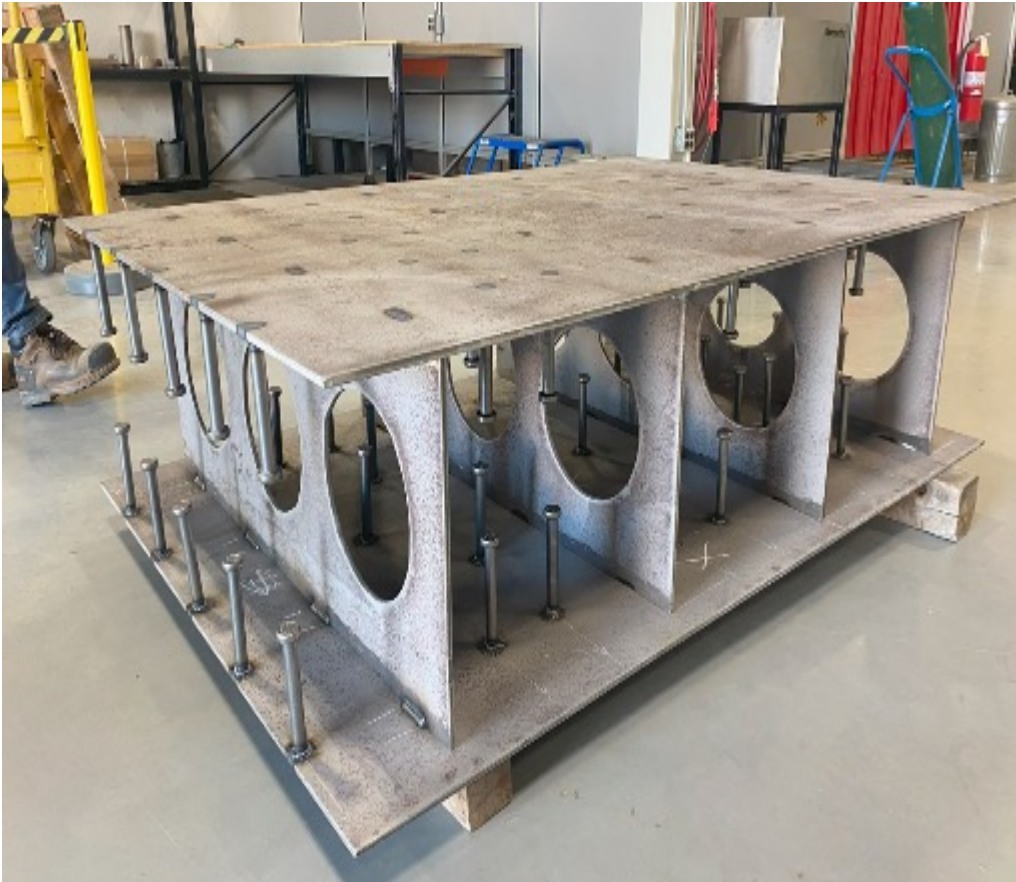
DPSC Scale - Model Wall Fabrication
