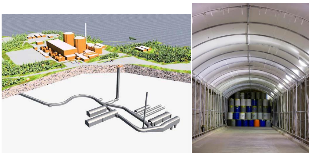
Figure 8-15. Loviisa LLW disposal facility. Cross-sectional view of the facility, including the planned extension for decommissioning waste (left) and, b) drums of LLW from reactor operation waste in the disposal hall (right). [Finland, 2020]
