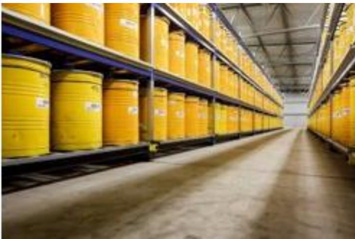
Figure 6-3. Interim storage of overpacked drums.
