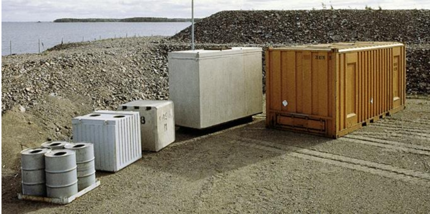
Figure 5-4. Different types of packages for LLW used in Sweden.
