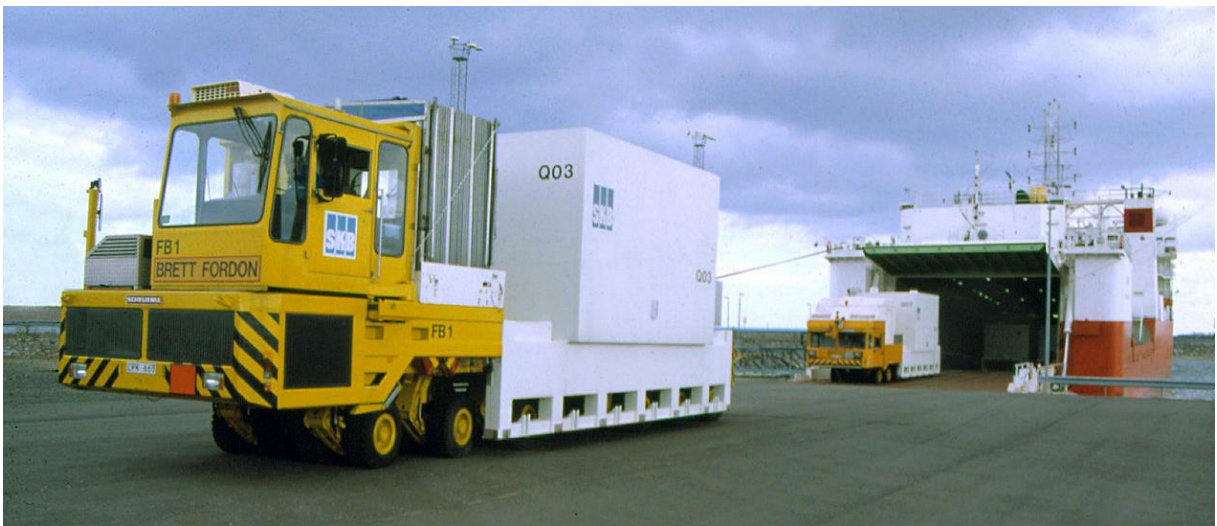
Figure 7-5. Loading of a transport container for LLW onto the Swedish ship dedicated for SNF and RW transports.
