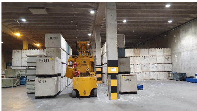
Figure E-4. Handling of waste packages in storage facility at Ringhals NPP.
