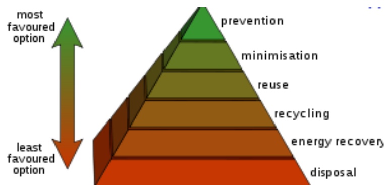
Figure 2.1. The waste management hierarchy to minimise the waste that will need disposal
