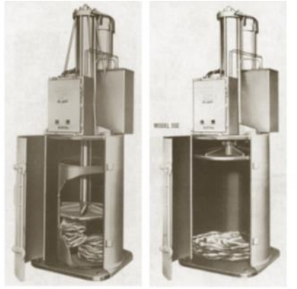
Figure 5-2. Simple compactor installation for in-drum compaction of VLLW.
