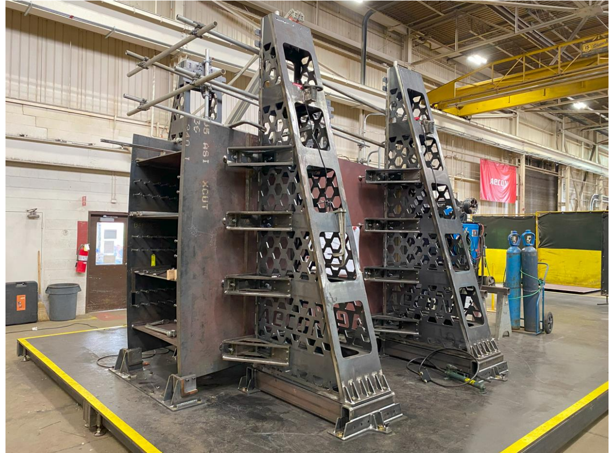
Basemat Prototype with Fixturing – Full Scale Fixturing Controls and Limits Distortion from Welding
